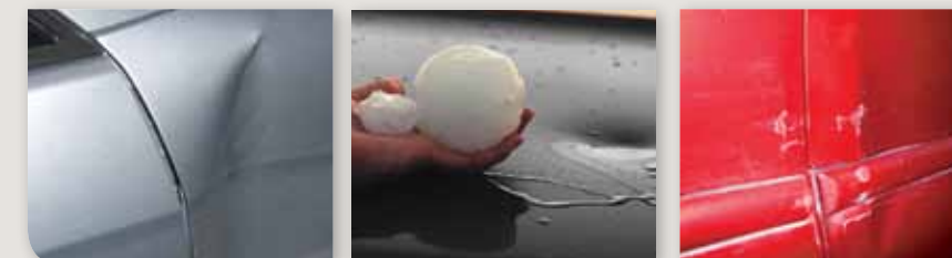
COLLISION DAMAGE HAIL DAMAGE PAINT SCRATCHES
